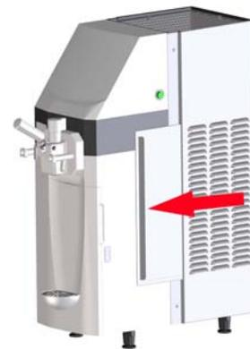
Remove the dirt and dust from the filters and replace the filters on the machine.
